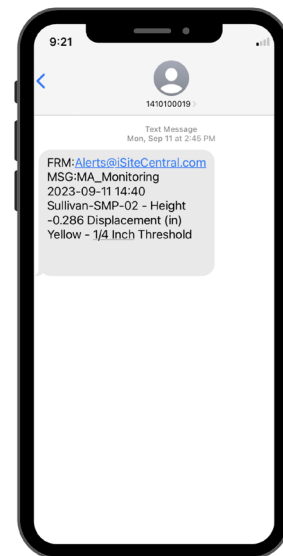
Mobile automated alert from sensor threshold exceedance
