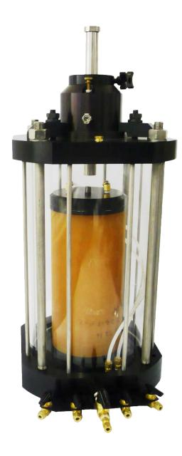
The Model 3600 is designed for triaxial, stress path, and resilient modulus testing of samples up to 150 mm (6 in.) diameter. It can also be used for flexwall permeability testing of samples. The chamber is acrylic with a circular base, which provides a solid support for applying heavy load and also prevents tipping. The outside diameter is 267 mm (10.5 in.) and the inside diameter is 241 mm (9.5 in.). All aluminum parts are anodized.
