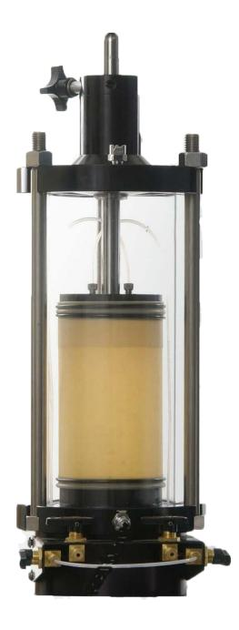
The Model 3500 is designed for triaxial and stress path testing of samples up to 100 mm (4 in.) diameter. Double drainage lines for both top and bottom allowing more flexibility and versatility.
