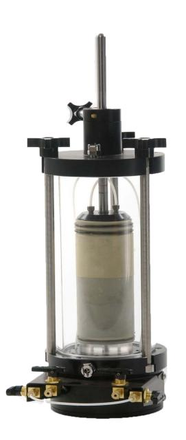
The Model 3400 is designed for triaxial and stress path testing of samples up to 76 mm (3 in.) diameter. It can also be used for flexwall permeability testing of samples up to 101 mm (4 in.) diameter. The chamber is acrylic with a circular base, which provides a solid support for applying heavy load and also prevents tipping. All aluminum parts are anodized.
