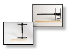
Dynamic Concrete Strain Gages (CSG) - measure axial strain in rigid pavement under long-term static (slab curling) or high-frequency dynamic (pavement response to trafficking) conditions. These ruggedized sensors are built to withstand the harsh conditions of concrete placement and vibration.
