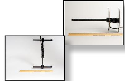
**Dynamic Concrete Strain Gages (CSG)** - measure axial strain in rigid pavement under long-term static (slab curling) or high-frequency dynamic (pavement response to trafficking) conditions. These ruggedized sensors are built to withstand the harsh conditions of concrete placement and vibration.
