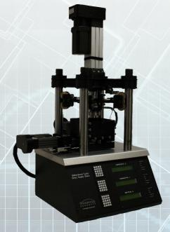
**Advanced or Bidirectional Cyclic Direct Simple Shear** Cyclic Direct Simple Shear ASTM D8296
