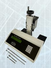
Lab Vane Shear System ASTM D4648
