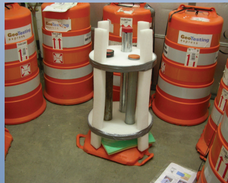
Invention of Shelby tube shipping container ('01)
