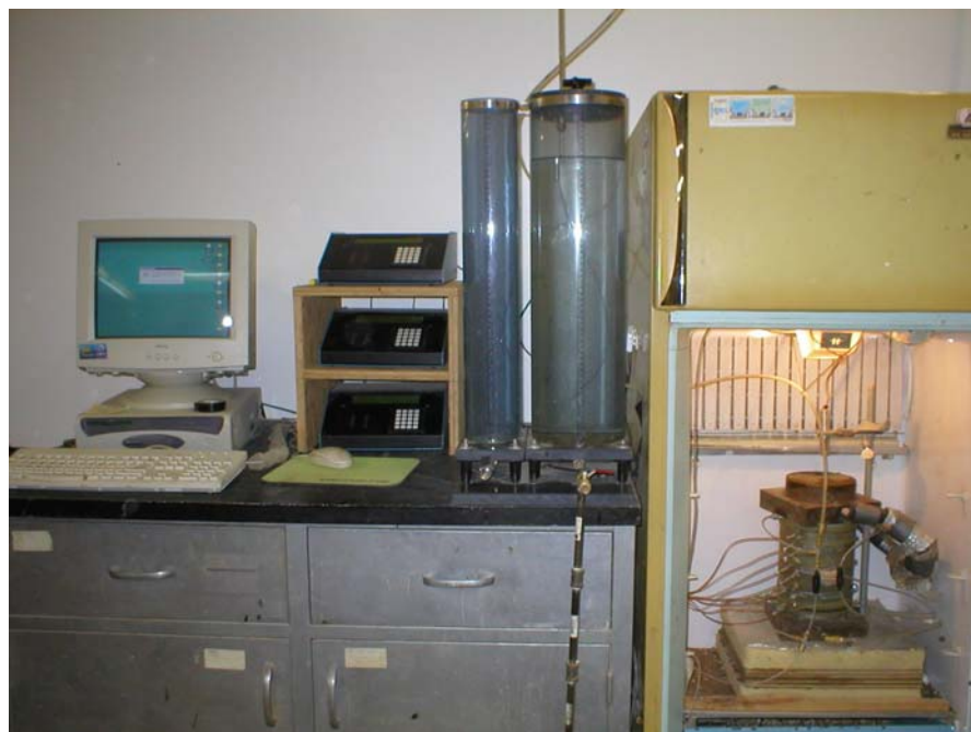
FIGURE 3—actual freeze-thaw / gas permeability test cell.
