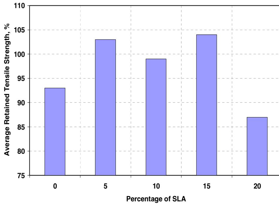
**FIGURE 6** Plot of average retained strength versus percentage of SLA in mix.
