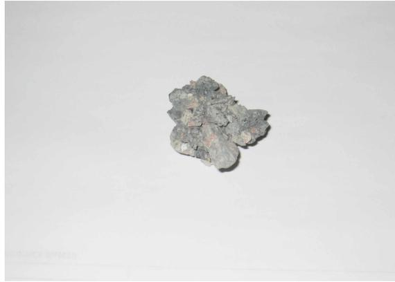
**FIGURE 2 Ball of (dry) aggregate and SLA.**
