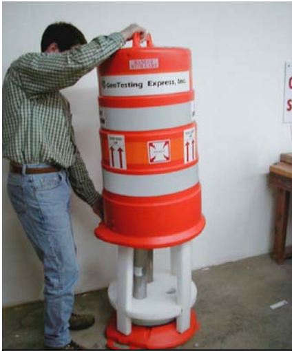
Fig. 4 Placing Barrel over Packing Insert
