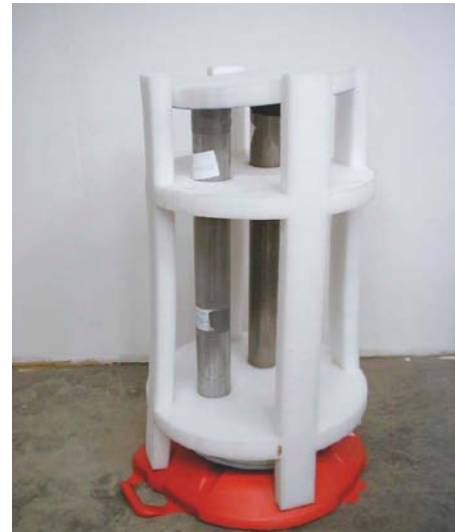
Fig. 3 Packing Insert with Shelby Tubes and Packing Top
