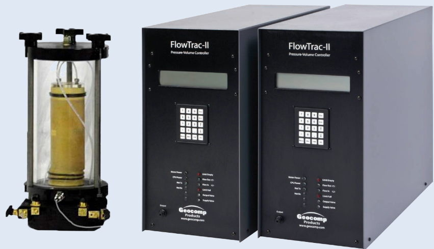
Standard Semi-Permeability FlowTrac II System
