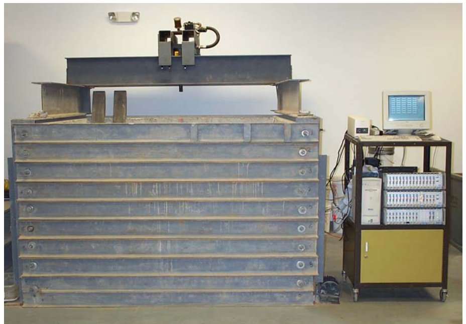
Full-scale pavement test box
