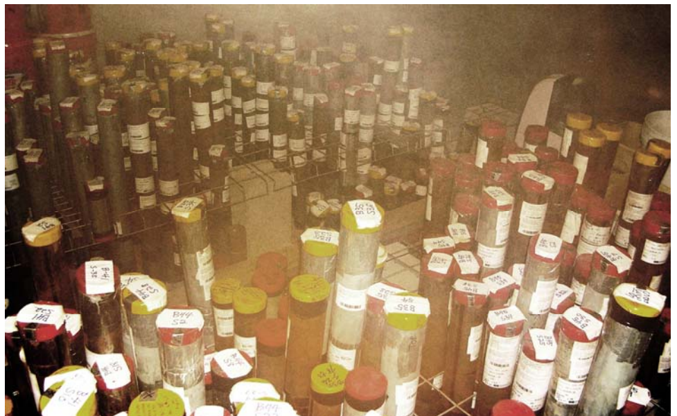
Shelby tube samples in the 100%-relative-humidity chamber
