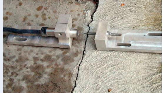
Prior to joining the bridge to the tunnels, a series of cracks were noticed in the concrete bridge deck. The cracks appeared in only a critical area of the bridge and inferred the possible presence of excessive tensile stresses in the concrete. The CA/T team performed non-destructive sonic testing that indicated the presence of voids in the concrete near the observed cracks.
